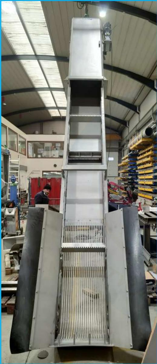
**REJA DE DESBASTE AUTOMÁTICA INCLINADA O VERTICAL CON DESCARGA AGUAS ABAJO PARA CAUDAL HASTA 25.000m<sup>3</sup>/h**
